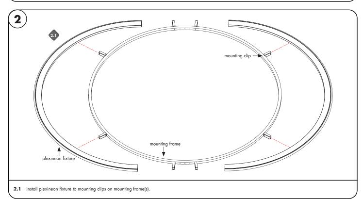
Models: Plexineon Vertical Rings Catenary Mount Static Color
