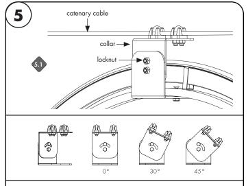
Loosen the top locknut on back of the collar to adjust the angle of plexineon fixture.
